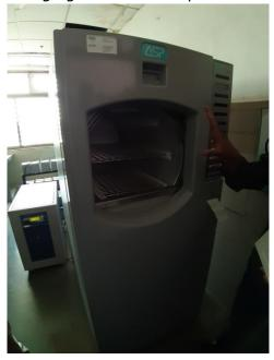
First the  $H_2O_2$  is inserted into sterilizer where it is heated at high temperature and is converted to gas and after that this gas is surrounded by an strong electromagnetic field as a result it becomes a plasma.
